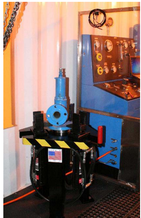
Valve Tester console with laptop, and test fixture (below)
