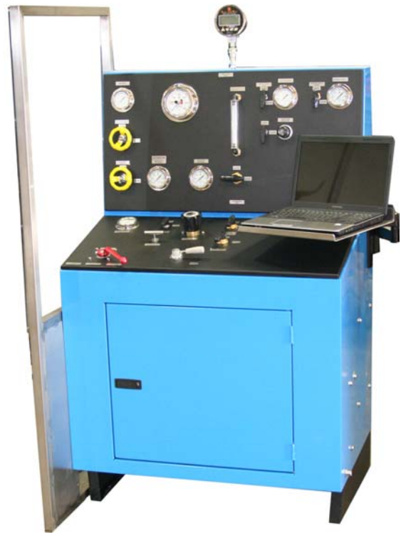
Valve Tester console with laptop, and test fixture (below)
