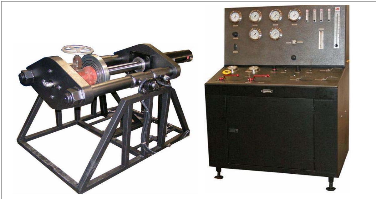
MODEL TF-100 T SHOWN WITH FIXTURE IN THE HORIZONTAL POSITION, CONTROL CONSOLE WITH BUILT IN RESERVOIR INSIDE, ALONG WITH HYDRAULIC POWER UNIT AND HYDROSTATIC PUMPS.
