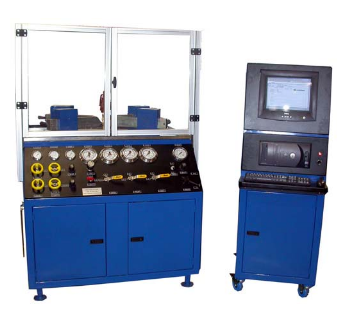
Model SRV Series shown with the optional Data Acquisition Console, for both relief and standard valves.
