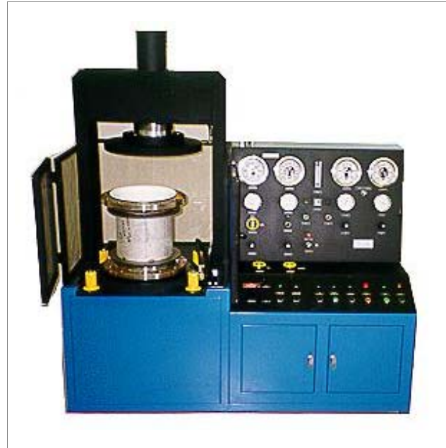
LVR Series shown with a 12" flanged turbine meter being tested.
